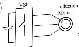
A 3-phase Voltage Source converter drives an induction motor load. The motor draws 2 MW active power and 600 kW reactive power at steady state operation. The motor terminal voltage is 6.6 kV (line to
