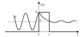
(b) Two copper nanowires are insulated by a copper oxide nano-layer that provides a 10.0 eV potential barrier. Estimate the tunnelling probability between the nanowires by 7.00 eV electrons through a 5.00-nm thick oxide layer. (5+2)
